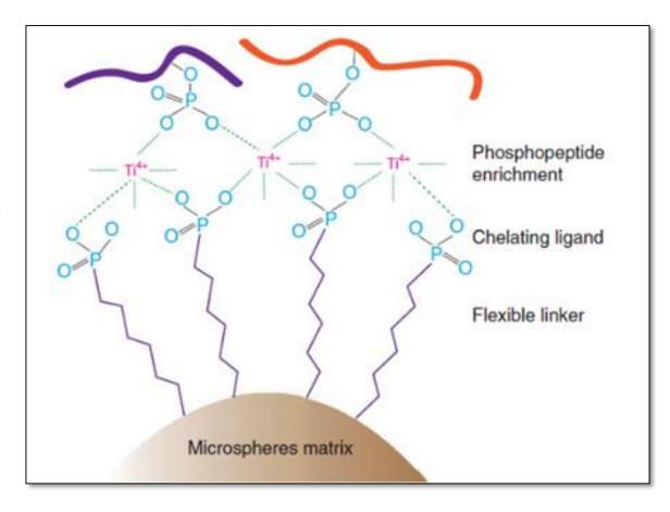
• In the last step, the elution of the captured phosphoproteins is made. Phosphoprotein/phosphopeptide - loaded Ti(IV) - IMAC sorbent is transferred to the elution medium and the phosphoproteins are separated from the surface.
